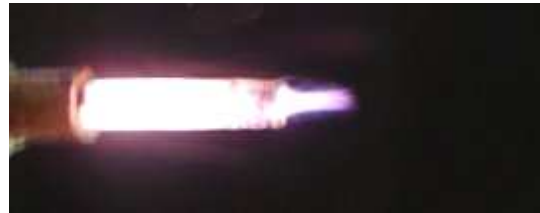
Fig.12 Ar-plasma jet in atmospheric pressure, experimentally observed in Faculty of Physics [26]
